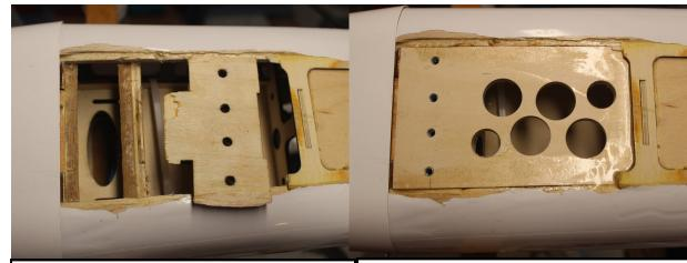
Dennys Stuff The above photo shows the landing gear structure of my "Revolver" model airplane. That LG plate pulled out of the fuselage after a very smooth landing, while a turn was made using the rudder.
