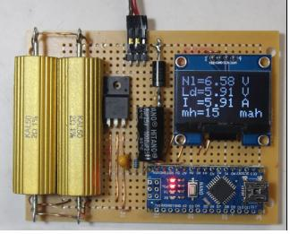
Note the display on this unit. It is showing the voltage of the battery under no load, the battery voltage under load, the actual discharge current, finally the total milliampere hour capacity discharged to this point. The test current is six Amperes, a current value that matches the currents pulled by our servos in our larger models.
