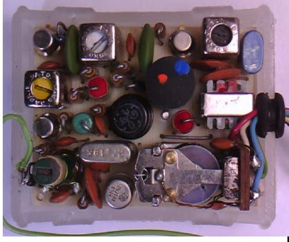
used "Stand Up" components that were very vulnerable to vibration breaking off the leads of the electronic components. Failures were common, and for my models, the average mean time between radio failures and crashes was less than 100 flights.
