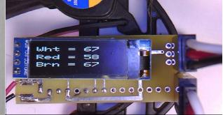
The left photo shows the 3D printed panel for the SwitchIR meter. Note the various cut outs for the OLED display, the servo connectors and the push button switch. There is even a compartment for the 9 Volt battery.
