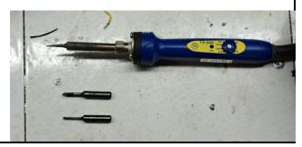
The Hakko iron allows the user to set the temperature of the iron tip to anywhere you'd like. And, since the tips do not overheat, they do not burn up, so they will last a long long time.
