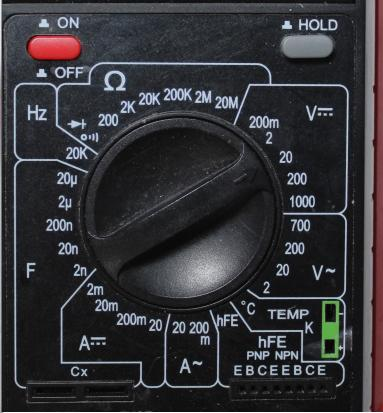
Right off the bat, we can scratch off the "F" and "hFE" functions. Those are electronic functions. F is a measure of Farads, or the capacity of a capacitor. hFE is the gain of a transistor.
