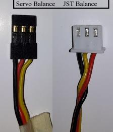
packs such as the LiPo's, LiFe and A123 packs use a white "JST" connector for the required balancing of the cells during the charge cycle.
