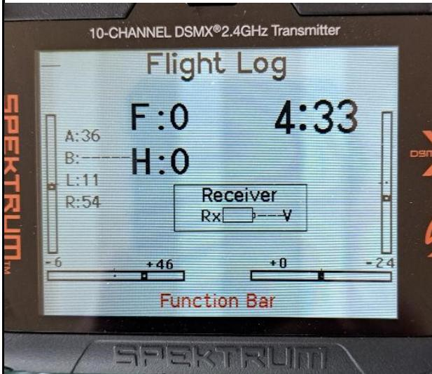
FYI, this is a photo taken of Hoss's new Spektrum nX10 transmitter immediately after landing, and before shutting off the receiver in the model. The 4:33 is the time left on the built in transmitter timer.
