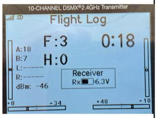
The photo above shows the nX10 information after a 6 minute flight on my Escapade model, built in 2015. Note that the receiver had 18 errors, the remote had 7, and the receiver lost both signals (Fades) 3 times during the flight. That three times represents a total of about 0.04 seconds out of the 6 minute flight.
