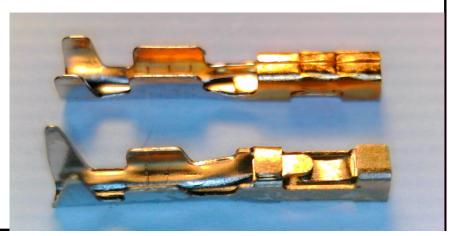
The top photo is the Maxx Products line, the bottom photo is the Amazon product. I checked contact resistance on both connectors. Both measured around 6.5 MilliOhms, a very low value indeed.
