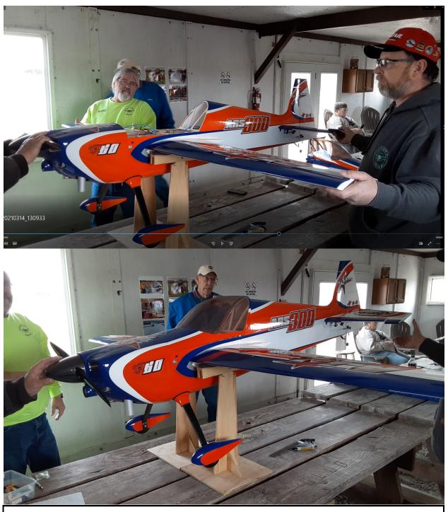
Note the very nice balancing setup for balancing this model. It looks to have been built up using standard 1/4 inch aircraft plywood, and a couple of narrow strips of bass wood or something similar. Nice set up.
