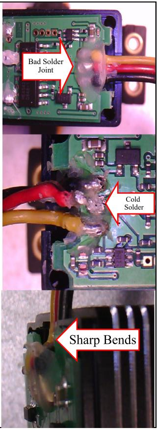
The manufacturing assembly process then in a \$150,000 expense to our supplier. placed the rubber material over the soldered connection, hiding the cold solder Any RTV that is safe for electronics equipioint.
