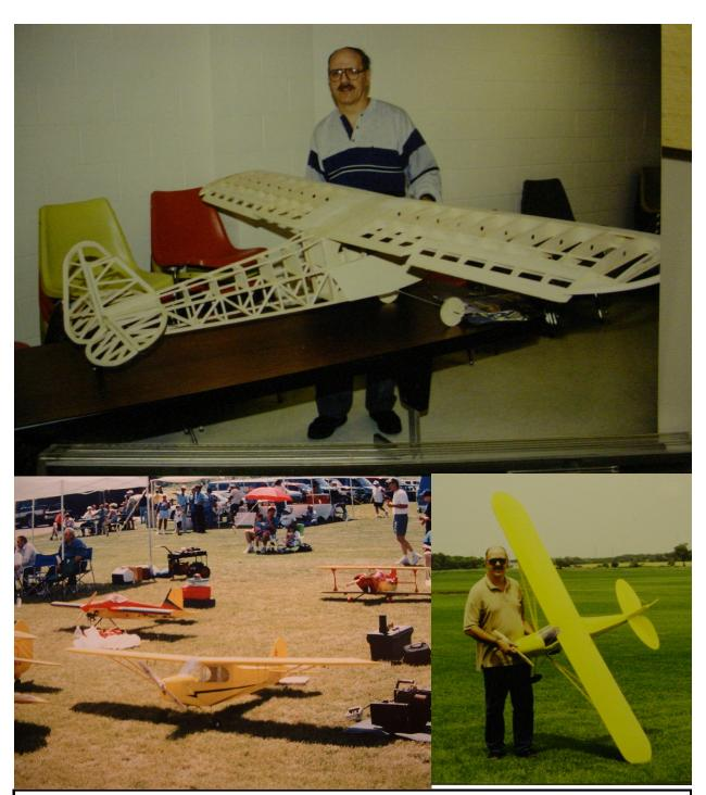
This is a 10 foot wingspan Piper cub your editor built over a 3 month period in 1999.. Power was an Astroflight geared 90 motor, and 36 SubC Nicad cells! It flew well, and it was flown at an all electric funfly in Allentown PA the following year.
