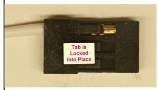
Use the modified jewelers screwdriver to push the terminal fully into the housing. Make certain that the tab has locked in the terminal.
