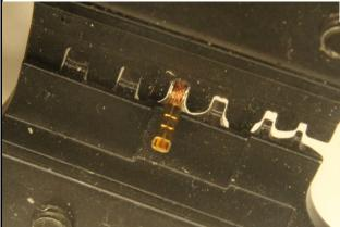
Next, **SLIGHTLY** crimp the terminal using the 1.6 mm jaws of the Engineer PAD -11 crimping tool. Just crimp the terminal sufficient to close the wings to where they just touch each other. Do not completely crimp the wire just yet.
