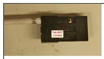
Next, insert the lead wire into the connector housing. Watch wire location!
