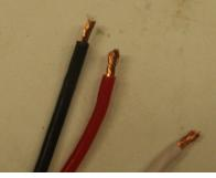
lation such that the bare leads will fill the wire crimping area of the terminals.
