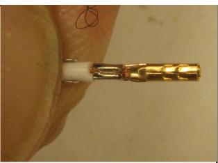
Now, move the terminal to the 1.3 mm jaws of the crimping tool, and fully crimp the terminal around the copper wire strands.
