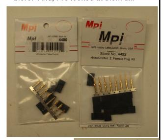
Starting off, Cut the pins out of the pin strips as shown to the right. Leave the rectangular tabs on the terminals to make a little "Handle" to hold the terminal and wire assembly while crimping the units.
