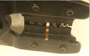
Finally, crimp the wire insulation restraint around the insulation of the wire. Slightly crimp with the 2.2 mm jaw, move to the 1.9 mm jaw, crimp a little more, and finish with the 1.6 mm jaw. The terminal
