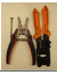
The orange handled tool is the Engineer PAD-11 crimping tool. Amazon has it for \$65.00. The wire stripping tool was found at Menards, Home Depot or Ace Hardware. Don't scrimp on either of these two tools. Not worth it. You also need a magnifying visor to see what you are doing.
