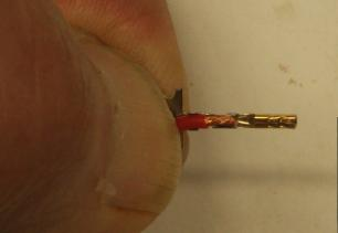
Hold the pin and wire as shown, making certain that the lead wire strands are below the wings of the terminal, and are centered in the crimping area.
